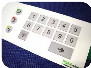
SENDING STATION (TOP) & KEYBOARD TO SELECT RECEIVING STATION CODE (BELOW)
